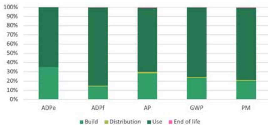
Figure 5 – Distribution of each life cycle step impacts for all environmental indicators.
